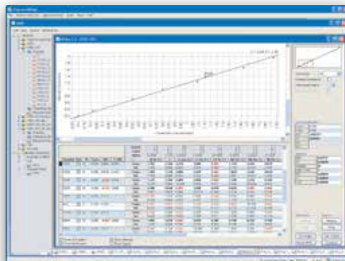
MVR calibration curve: real concentrations vs. intensities
