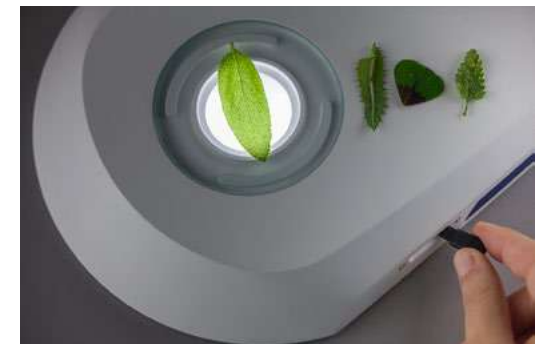
Use the flat transmitted light unit to contrast colored transparent specimens in bright- and darkfield. Add polarizer/analyzer equipment to observe, for example, birefringent crystals or tensions in glass or plastics.
