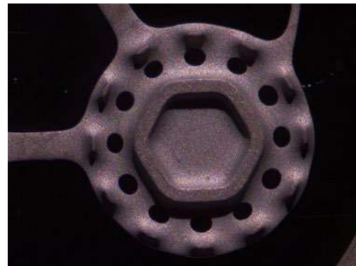
Automotive component; spot K LED, oblique light, zoom 1.5x, front optics 0.75x
